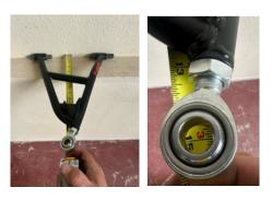
Step 8: Install the lower arm back onto the bulkhead but leave out the 15mm bolt in the front until you have completed the second side. This bolt goes through both sets of arms. Use the supplied bolt for the lower shock mount and the supplied bolt for the lower sway bar mount. The sway bar dogbone goes on the outside of the tube closest to
