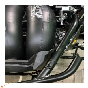
Start the 2 Allen bolts loosely into bumper, the bolts in center support bar, the bumper to nose cone bolts, and the lower torx, once all started then go back and secure all the bolts.
