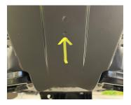
**Step 4:** Drill ¼ hole for support bracket bolt. There is an indented diamond molded into the nose cone that marks the correct spot to drill. Install the new lower support bracket and lower bolt but leave it hand tight.
