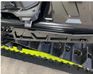
Step 4: Fit side supports into place using (3) short rivets on each side placed into the factory holes. Install the rear bumper section using (2) of the long rivets. Once you have everything aligned and in place use your rivet tool and install the rivets from front to rear.
