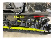
**Step 2:** Remove the reflector and track length sticker. A heat gun helps warm everything up and can make it easier to remove. If there is any residue you can rub it with your finger and it will come off. Be careful not to damage the paint!
