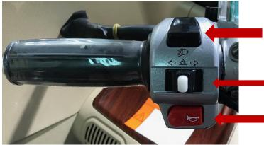
High beam & low beam switch
