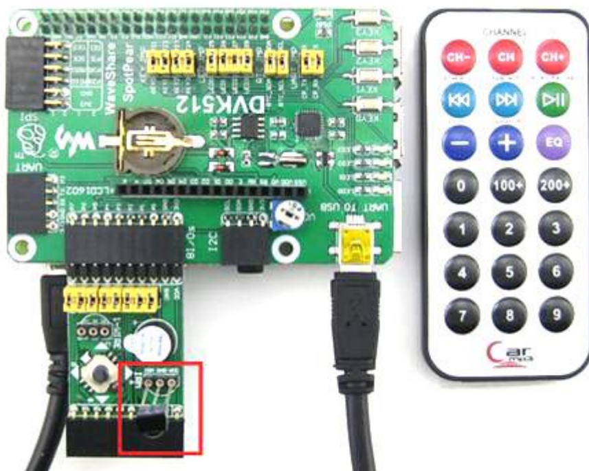
Figure 5: Connecting the infrared receiver to the IRM interface on Mix Board
