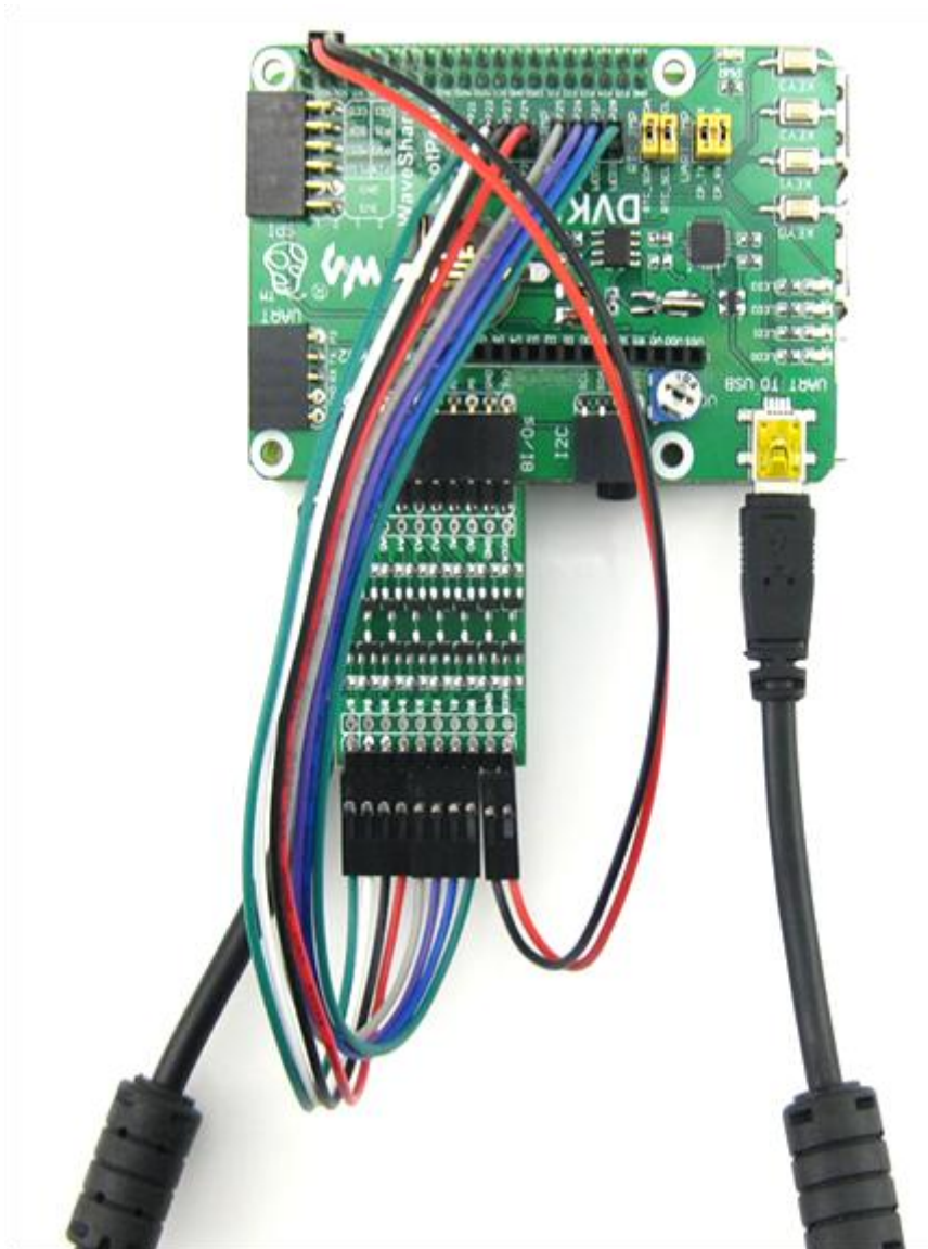
Figure 3: The Connection between Logic Level Converter and DVK512
