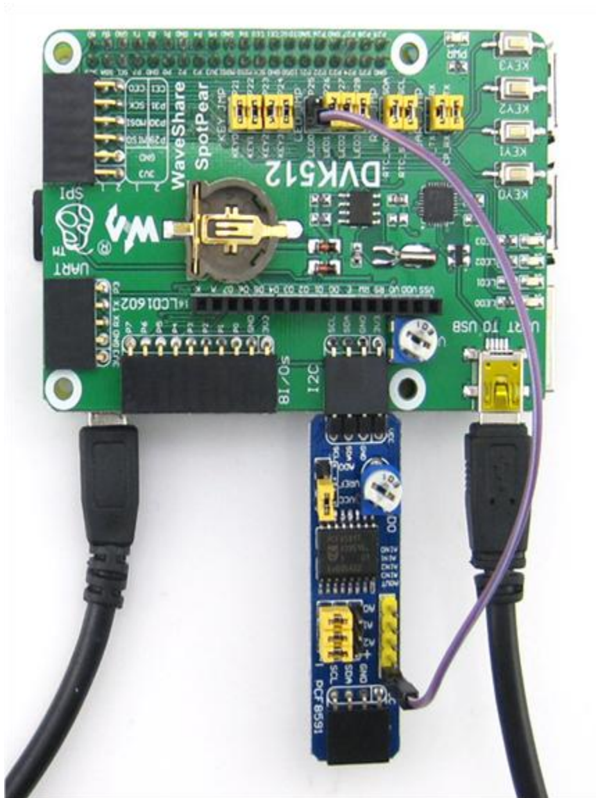
Figure 11: Connecting the Pin AOUT on PCF8591 to the LED pin header on DVK512
