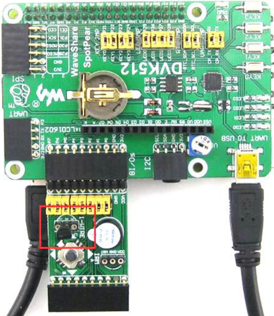
Figure 4: Inserting the DS18B20 to the ON-WIRE interface on Mix Board
