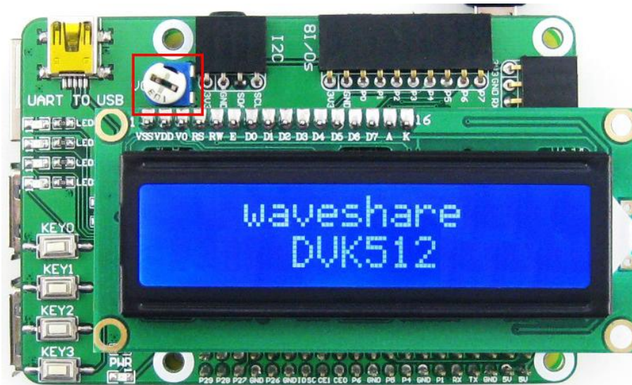
Figure 7: Inserting the LCD1602 into the LCD1602 interface on DVK512
