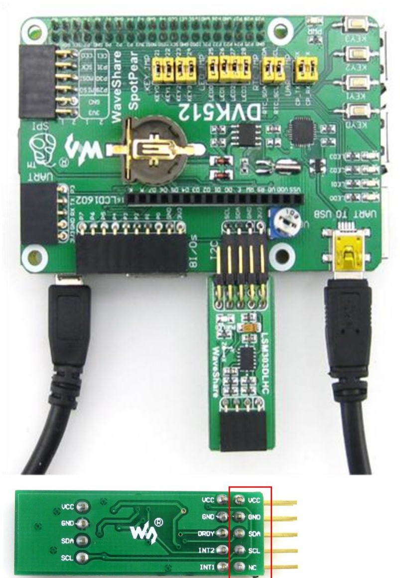
Figure 12: Connecting the LSM303DLHC module to the I2C interface on DVK512
