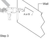
Marked 2 dots on wall with length of A or B, and drill holes
