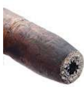
Nozzle fully clogged (not using E-WELD Nozzle)
