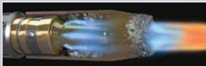
Spatter build up obstructs gas flow, resulting in inconsistent weld quality.
