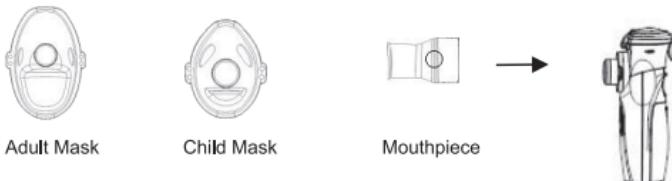
**Figure 5 Fitting the accessories**
