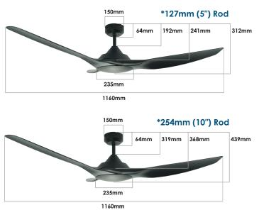
\*Supplied with: 127mm (5") Rod and 254mm (10") Rod
