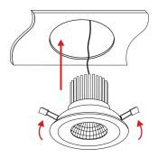
Bend springs upward and install luminaire into ceiling.
