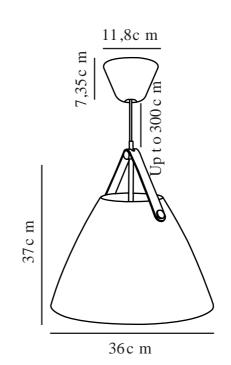
Voltage (V): 230 Volt IP degree: IP20 Maximum bulb wattage (W): 40W Class (Class 1, Class 2, Class 3): Class 2 (Double isolated) Socket type: E27 Dimmerable: Yes with compatible bulb
