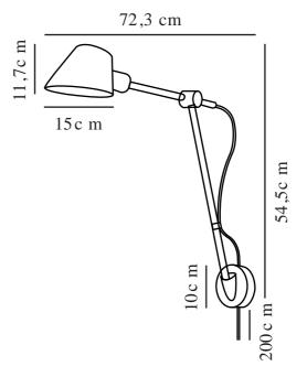
Voltage (V): 230 Volt IP degree: IP20 Maximum bulb wattage (W): 60W Class (Class 1, Class 2, Class 3): Class 2 (Double isolated) Socket type: E27 Switch placement: On the fixture
