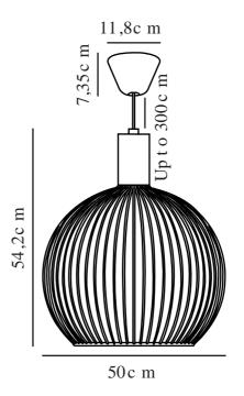
Voltage (V): 230 Volt IP degree: IP20 Maximum bulb wattage (W): 60W Class (Class 1, Class 2, Class 3): Class 2 (Double isolated) Socket type: E27
