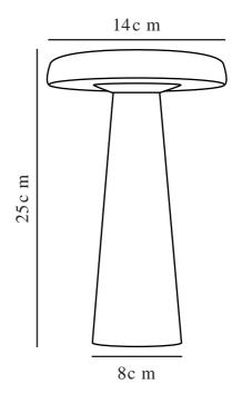
Voltage (V): 220-240 Volt IP degree: IP54 Class (Class 1, Class 2, Class 3): Class 3 (12V) Socket type: LED Module Switch placement: Under the base
