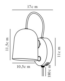
Voltage (V): 230 Volt IP degree: IP20 Maximum bulb wattage (W): 25W Class (Class 1, Class 2, Class 3): Class 2 (Double isolated) Socket type: GU10 Switch placement: On the fixture
