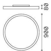
Net weight 6.9 kg Insulation class I **Protection index** IP40 Compliance CE Operating temperature 0° ~ +40 °C
