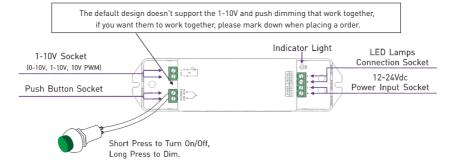
12V lamp connected, loads 0~144W(12V).
