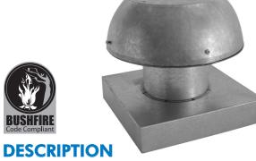
The Ezifit Roof Series, with bushfire code compliance, has been developed and tested for exhaust air applications in bushfire prone regions. They are driven by a high performance centrifugal fan and have a low profile design. They can exhaust from a number of points within the building and are available in 150 and 200mm fan sizes.
