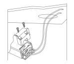
Step 3 Connect the downlight with driver, hold back the spring clip then push the downlight into the hole.
