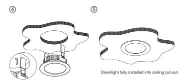
Fold spring clips and push into cut out.
