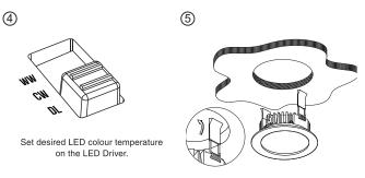
Fold spring clips and push into cut out.
