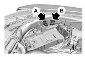
There are three sets of blunt-cut and sealed circuits. Two sets are under the hood and behind the battery tray, and one set is inside your vehicle at the passenger footwell.
