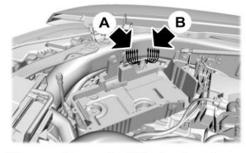
There are three sets of blunt-cut and sealed circuits. Two sets are under the hood and behind the battery tray, and one set is inside your vehicle at the passenger footwell.
