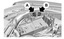
There are three sets of blunt-cut and sealed circuits. Two sets are under the hood and behind the battery tray, and one set is inside your vehicle at the passenger footwell.
