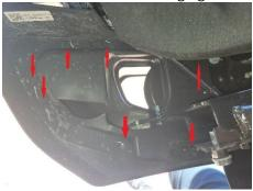
With the cover off please remove the wiring harness clips and final 4 bolts which hold the OEM fog light in place. Unclip the main harness from the fog light and remove the unit from the bumper.
