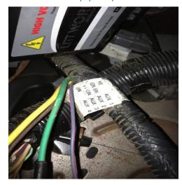
"The Bronco Nation" has a very educational video illustrating how and where the wiring is. They also show a way you can drill through to feed the wiring through the inside of the vehicle instead of running it on the outside along the window into the engine bay. If you are running it down the window, we recommend using silicone to keep the wire in place.
