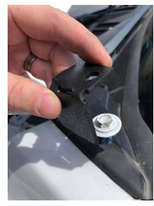
Install the bracket using the factory 10mm bolt.
