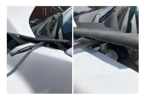
5. Apply Loctite 242 to the threads of the fender bolts and insert into bracket. Notice the curved part of the bracket, this should match the contour of your windshield.
