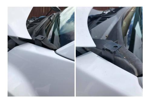
6. You can now grab the light pod assembly and bolt it to the bracket using the supplied hardware. Make sure to use Loctite 242 on the threads, and tighten with 2 13mm wrenches.
