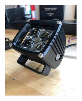
We suggest to only snug up the bolts for now. You will need to aim the lights once installed, and then tighten.
