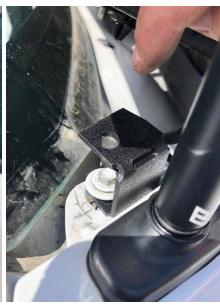
You should now be able to lower the wiper tray back into place, and flex the wiper tray around the light pod brackets. No cutting or modifications are required.
