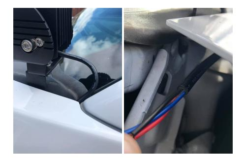
Attach a ring terminal to the black wires and attach them to a good chassis ground or the battery ground. Add wiring length as needed with the barrel crimps and additional wire. The red and blue wires go to your upfitter switch wiring on the passenger side firewall. You can wire the amber halos independently or together on the same switch. Make sure to properly crimp all the connections and to tape up any exposed connections. We also suggest you cover the wires with wire loom.
