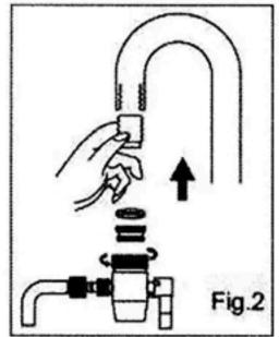
2. Fitting the Ceramic Element: Unscrew the Sump from the Base. Remove ceramic cartridge (Fig. A) from its protective Sleeve and plant it on to the base with the hole end. Do not Over tighten. Screw the threaded sump into the Base. Hand tighten only.
