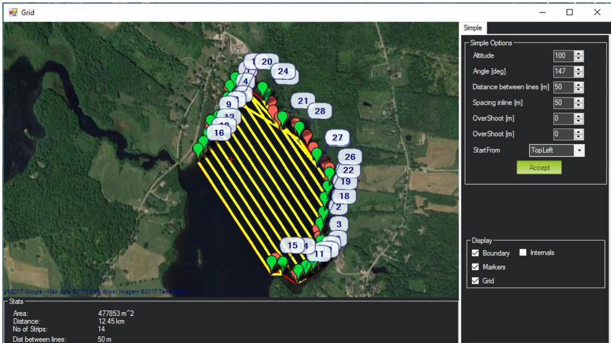
Please uncheck the “internals” box. You may also adjust the other parameters available to suit your needs. The most common and useful parameters are the “Angle” and “Distance between lines” which are self explanatory.
