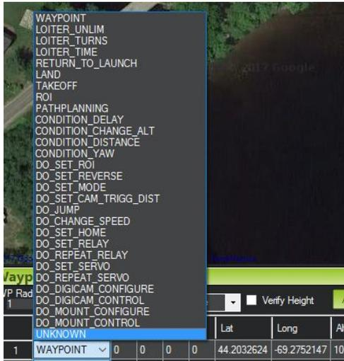
Each command has a drop down which allows you to specify the type of command. You can see an example of the functions available in that drop down menu to the left. Depending on the type of command selected, the four following boxes on that row may change to allow additional functionality.
