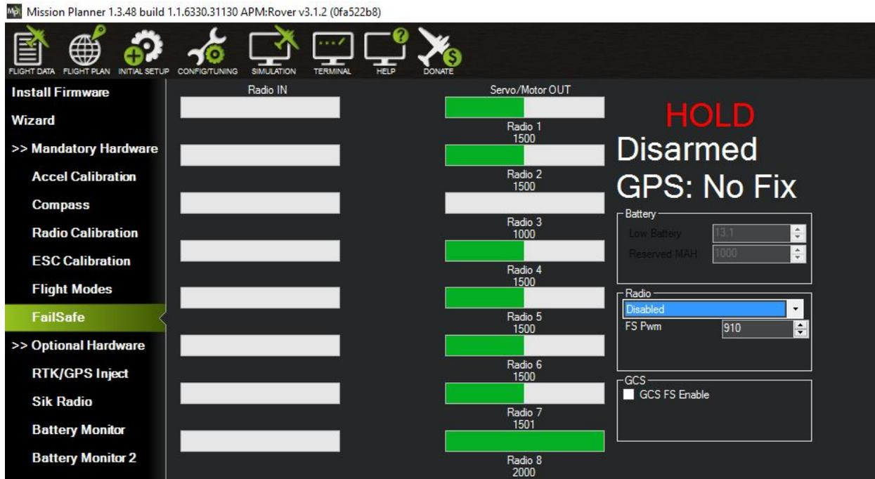
To set R/C Signal Loss Failsafe, navigate to Initial Setup tab => Mandatory Hardware => FailSafe as shown above.
