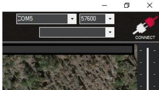
3. Once you have chosen the correct COM and BAUD Rate as described above, press "Connect." Mission Planner will establish a link to the SimpleSCAN and begin downloading the vehicle specific settings - this allows Mission Planner to understand the sensors and equipment on the SimpleSCAN (or other vehicles you may use)
