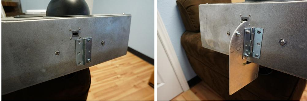
Once the rudder is securely attached, connect the servo control rod to the horn on the rudder. If you have trouble getting the clevis open, you may use a small flat head screwdriver to pry it, slip it onto the horn until the pin finds the hole and connects to the clasp on the other side.
