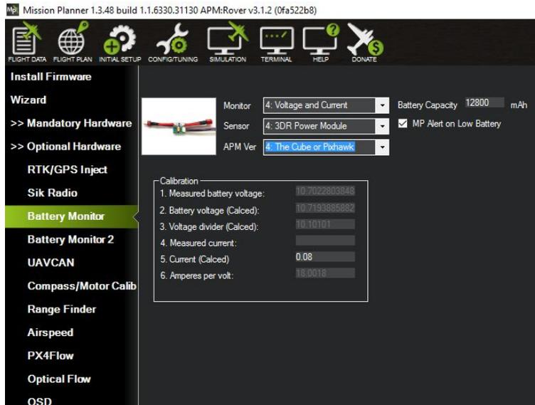
To adjust the current calibration, access the “Battery Monitor” section from the “Initial Setup” tab as shown above.
