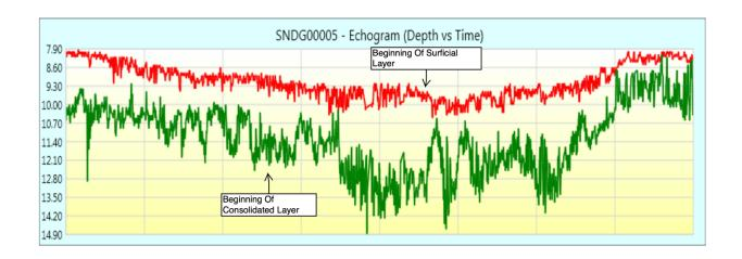
Typical echogram along a survey line as presented by HydroMagic™, HYPACK™, or similar PC-based Hydrographic Mapping Software.
