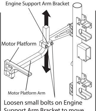
Loosen small bolts on Engine
