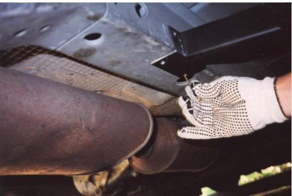
**5.** Next step is to drill out the 6 holes into the frame rail with the 5/16" drill bit, using the 1/8" bit to pilot the holes first. Again, double check to assure that everything is in the right spot before you start drilling. I've found that if you use the smallest drill motor you have, this seems to work
