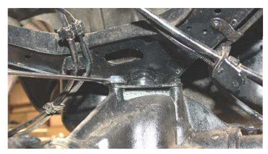
2) Remove the e-brake and brake line cable from the upper a-arm using a 10mm socket to allow the a-arm to raised enough to allow installation of a-arm spacer. Re-install the upper a-arm bracket using the supplied  $14mm \times 100mm$  (approx 4") bolts from Hardware kit. Tighten using a 22mm socket or end wrench.
