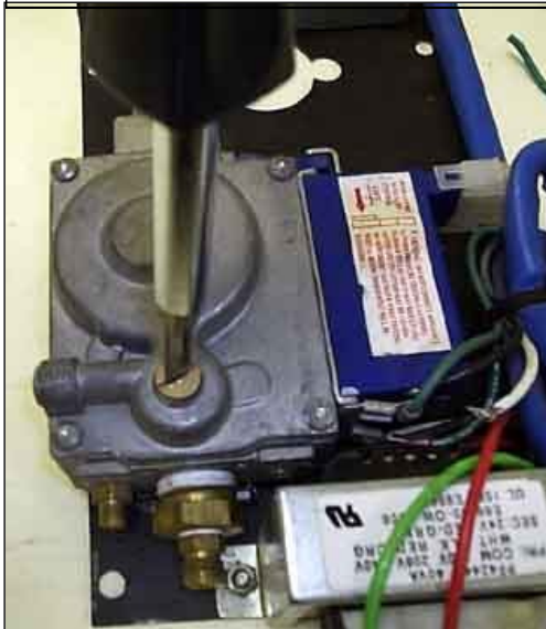
Photo 13. Inside view, adjustment screw.
