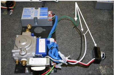
6. Remove the gas kit inner backplate by removing the hexnuts from the four inner holes as shown.
