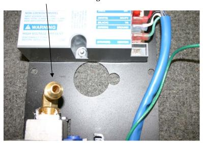
3. Loosen and remove the gas line and pilot line from the bottom of the gas valve. Be careful not to kink the gas lines.
