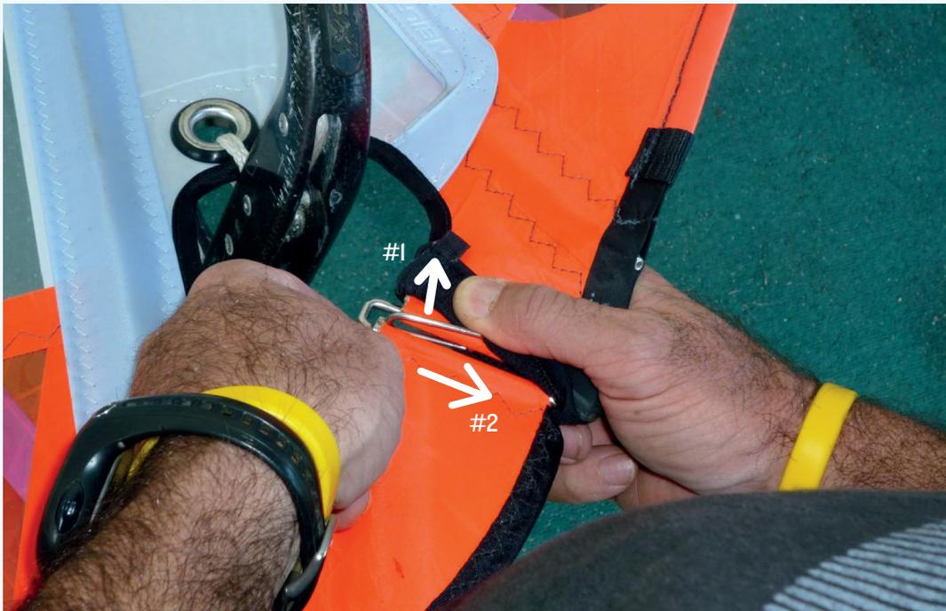
Then pivot and push to align the short end (pin) in the tube on the inside of the hole, use your finger on the bottom of the sail (back side) to help align them on the horizontal plain.
