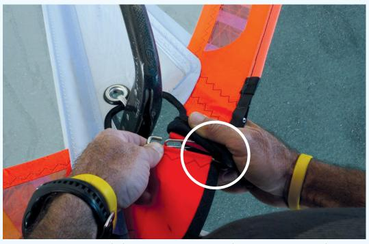
Engage the long end of the link (Pin) into the tube of the other half (leech side is first to engage) as shown on photo above.
