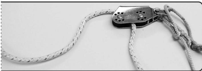
7. Take the rope back to the bottom 244BLK and feed the rope from the cleat side around the roller on the far side from the fixed attachment point.
