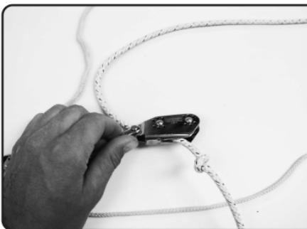
6. Loop the top 244BLK. Feed the rope from the cleat around the roller on the far side from the fixed attachment point.
