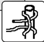
The next step will be to put it on the sail. Tie the 100 cm 4mm Spectra Rope around the mast with a Cow Hitch as shown on image.
