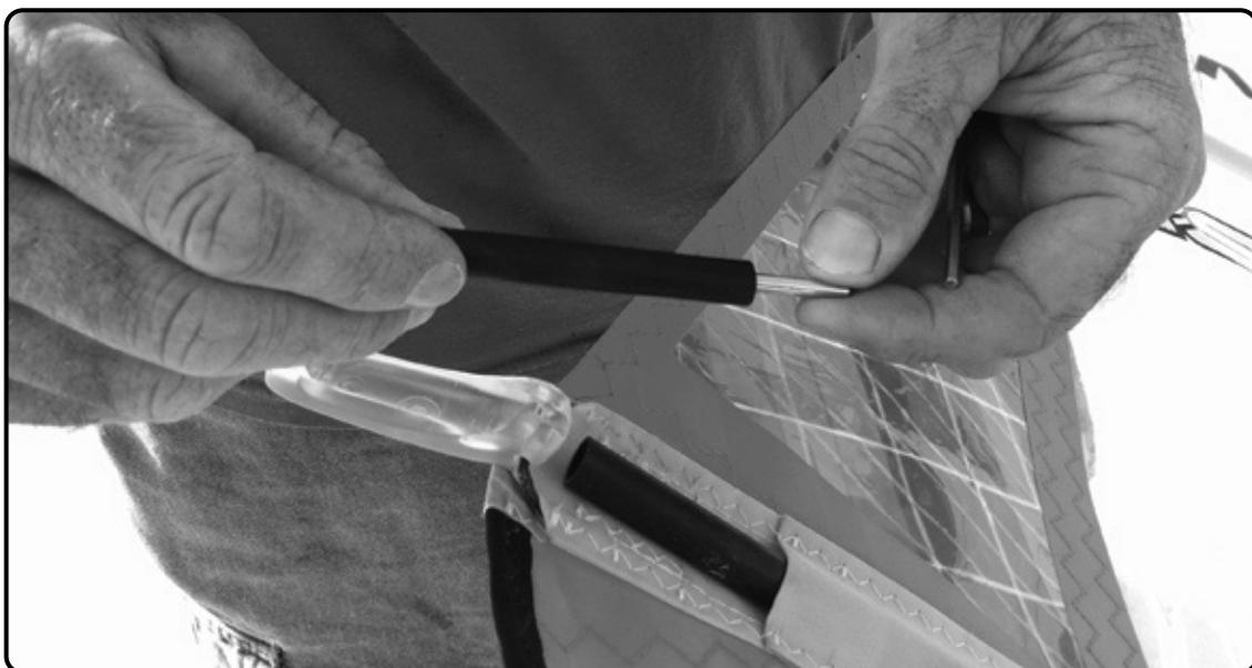
c. Slide the piece back into the batten and close the bat-cam. If it's too hard to close the bat-cam easily then please make the mechanism a little shorter to prevent possible damage to the bat-cam. As on the image below, the batcam will be too hard to close.
