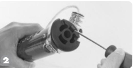
Using a small sc rew driver, pry the spring out
