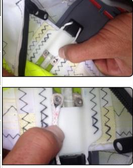
Slip the rope loop over the metal. The rope closest to the top of the sail goes underneath the sleeve material and the other rope goes above.
