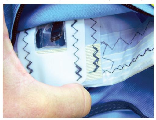
8. Grab the batten tip with some pliers and pull the broken part out of the sail.
