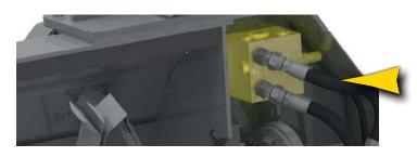
Bi-directional flow manifold with cross-over relief allows the operator to direct debris away from bystanders, other machinery, and buildings
