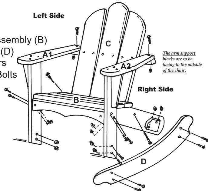
1. Please inspect all parts for damage during shipping and for any missing items. If you suspect that there may be damage or a shortage, call us and we will send replacement parts if needed. At this time, visualize how the components fit together per the above drawing and make sure that you have everything identified. You will need a standard Phillips screwdriver, a flat head screwdriver and a pair of pliers.
