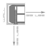
\*Bracket must be screwed into a stud for tested strength. Product tested on ½" gypsum board. Set screw tested to hold 125 lbs vertical and horizontal pull.
