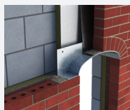
Parabolic Arch Lintel
