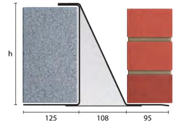
Standard lengths are available in 150mm increments up to 3000mm, 300mm at lengths 3000mm to 4800mm (including 4575mm, but excluding 4500mm).
