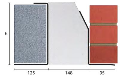
Standard lengths are available in 150mm increments up to 3000mm, 300mm at lengths 3000mm to 4800mm (including 4575mm, but excluding 4500mm).
