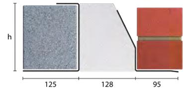
Standard lengths are available in 150mm increments.
