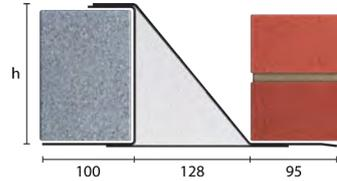
Standard lengths are available in 150mm increments.
