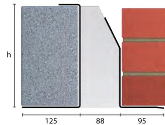
Standard lengths are available in 150mm increments up to 3000mm, 300mm at lengths 3000mm to 4800mm (including 4575mm, but excluding 4500mm).
