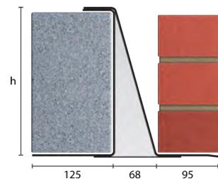
Standard lengths are available in 150mm increments up to 3000mm, 300mm at lengths 3000mm to 4800mm (including 4575mm, but excluding 4500mm).
