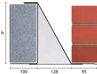
Standard lengths are available in 150mm increments up to 3000mm, 300mm at lengths 3000mm to 4800mm (including 4575mm, but excluding 4500mm).
