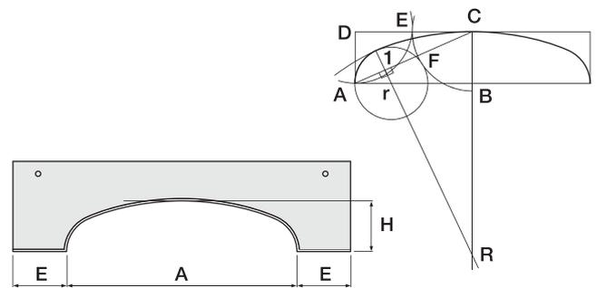
Draw rectangle  $ABCD$ . Make  $DE = DA$ . Make  $CF = CE$ . Bisect  $AF$  to make point  $1$ . Project a right angle off  $AF$  at point  $1$  to find small radius  $r$  and project further to find large radius  $R$ .
