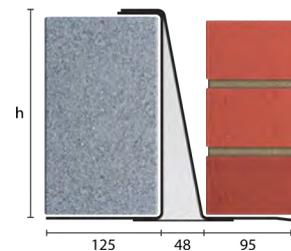
Standard lengths are available in 150mm increments up to 3000mm, 300mm at lengths 3000mm to 4800mm (including 4575mm, but excluding 4500mm).
