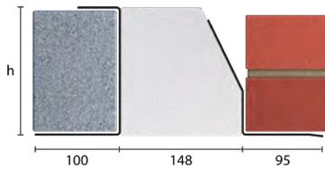
Standard lengths are available in 150mm increments.
