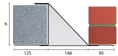
Standard lengths are available in 150mm increments.
