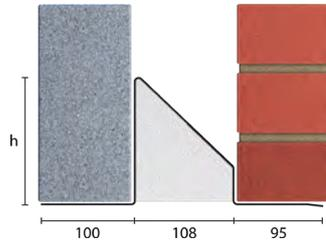
Standard lengths are available in 150mm increments up to 3000mm, 300mm at lengths from 3000mm to 3600mm.
