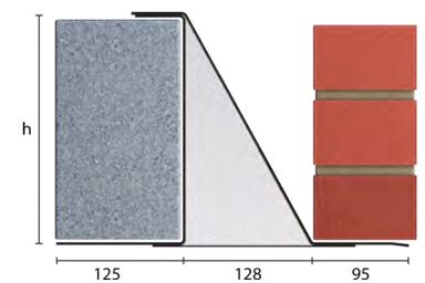
Standard lengths are available in 150mm increments up to 3000mm, 300mm at lengths 3000mm to 4800mm (including 4575mm, but excluding 4500mm).
