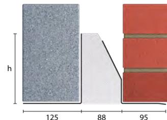
Standard lengths are available in 150mm increments up to 1800mm, 300mm at lengths from 2100mm to 3000mm.
