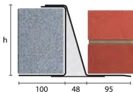
Standard lengths are available in 150mm increments.
