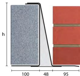
Standard lengths are available in 150mm increments up to 3000mm, 300mm at lengths 3000mm to 4800mm (including 4575mm, but excluding 4500mm).
