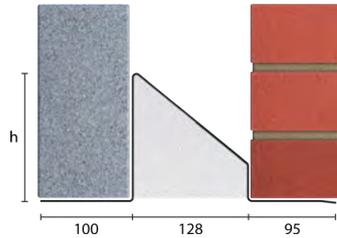
Standard lengths are available in 150mm increments up to 3000mm, 300mm at lengths from 3000mm to 3600mm.
