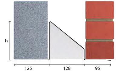
Standard lengths are available in 300mm increments.
