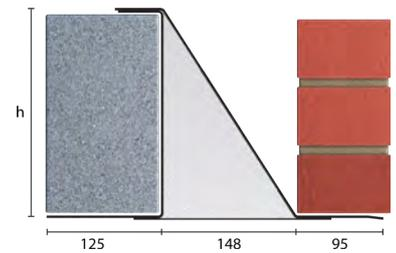
Standard lengths are available in 150mm increments up to 3000mm, 300mm at lengths 3000mm to 4800mm (including 4575mm, but excluding 4500mm).
