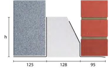
Standard lengths are available in 150mm increments up to 1800mm, 300mm at lengths from 2100mm to 3000mm.
