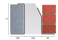
TX130/100 Standard lengths (mm) 750-2250-2850-3300-4200-2100 2700 3000 3900 4800 SWL 1:1/19:1 (kN) 60 60 55 50 32 Weight (kg/m) 17.0 21.9 21.9 21.9 21.9 Nominal height 'h' (mm) 229 229 229 229 229
