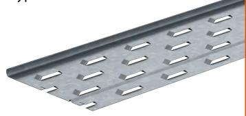
Manufactured from galvanised steel to BS EN 10346:2009 of grade Z275 the external plaster key provides a secure key for a rendered finish.
