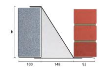
CX150/100 Standard lengths (mm) 900-2700 2850-3000 3300-3900 4200-4800 SWL 1:1/19:1 (kN) 60 55 50 32 21.9 Weight (kg/m) 18.2 21.9 18.2 Nominal height 'h' (mm) 232 232 232 232
