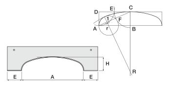
Draw rectangle ABCD. Make DE = DA. Make CF = CE. Bisect AF to make point 1. Project a right angle off AF at point 1 to find small radius r and project further to find large radius R.
