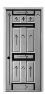
**RECOMMENDED:** Apply the Wood Grain Finish Coat over the Wood Tone Base Coat per the grain direction depicted in the images to the left of the page because it's the most common grain found in wood doors.
